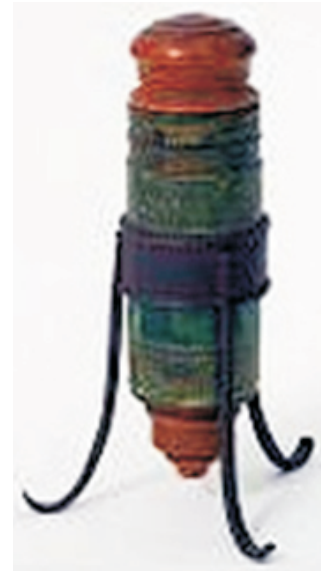
Figure 2. Galileo Galilee develops a compound microscope with a convex and a concave lens
